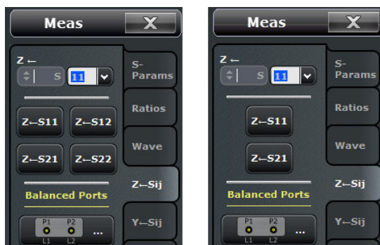
left = R&S ZNC or bidirectional R&S ZND right = unidirectional R&S ZND
