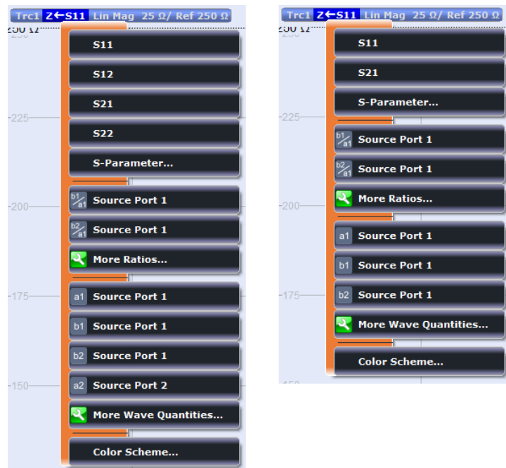
left = R&S ZNC or bidirectional R&S ZND right = unidirectional R&S ZND
